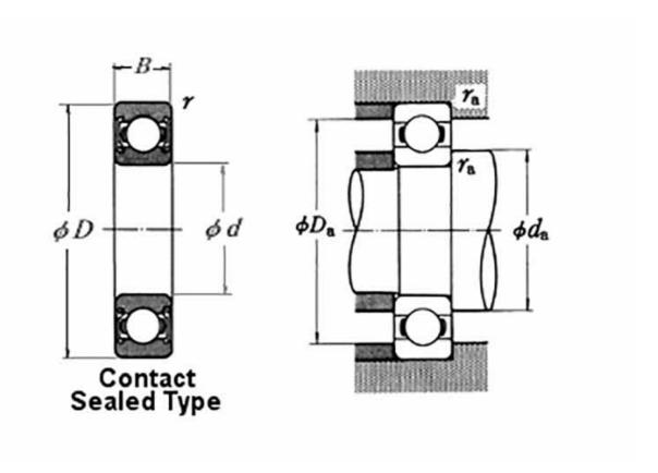
High quality Deep groove ball bearing with rubber contact seals from the world leader NSK, the worlds largest ball bearing manufacturer offering unparalelled quality. The unique & patented NSK DDU rubber seal features market leading technology, keeping contaminants and moisture out of the bearing while retaining the high class lubricant inside
